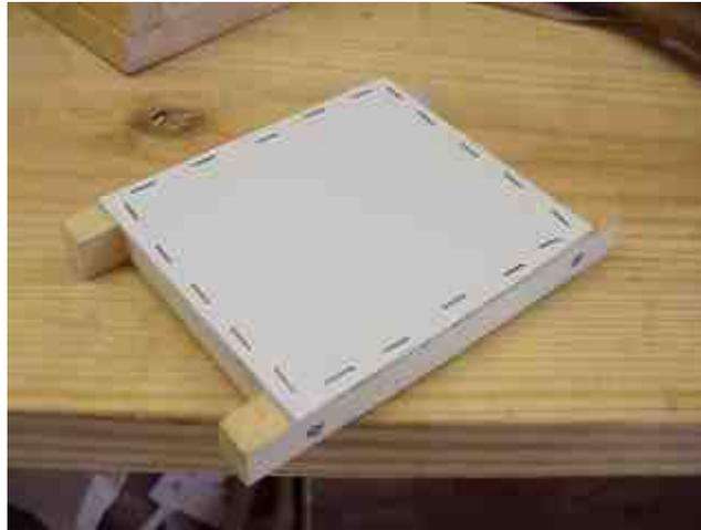
Seal the styrene around its edges with masking tape. The idea is to get as air-tight a seal as possible.
