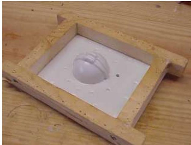
Remove the styrene from the frame.
