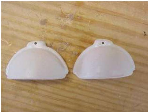
Sand the blinker surfaces with 60 grit sandpaper to roughen the surfaces to receive paint.
